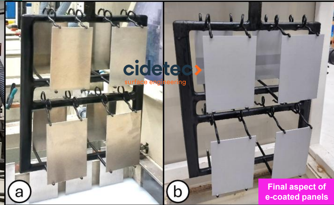
Aluminum test panels (AA2024-T3) before (a) and after (b) electrophoretic lacquering.
